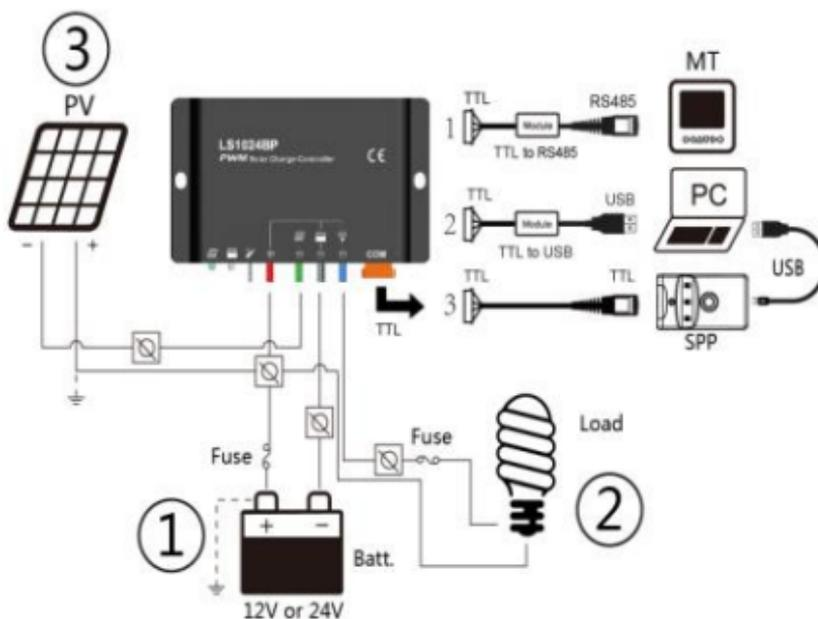
1. Connect components to the charge controller in the sequence as shown above picture and pay much attention to the “+” and “-”. Always power the battery First.
